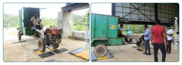
Figure 16: Weighing the unloaded vehicle
