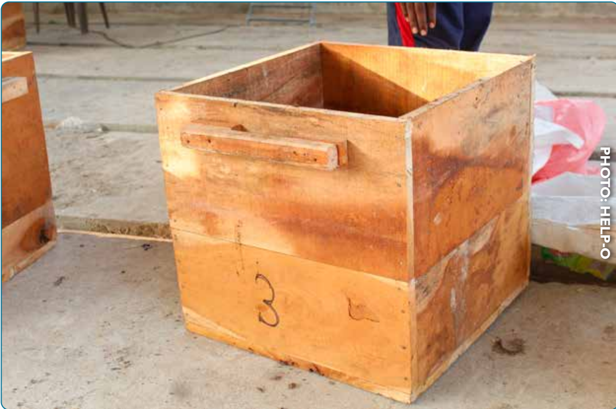
Figure 12: Wooden Box for taking the volume of the waste
