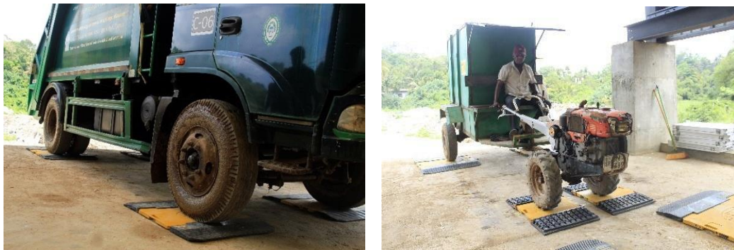
Figure 6: Weighing the Waste Collection Vehicle Fleet of the GMC (Source: WACS Report, 2023)
