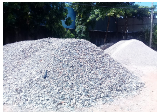
Figure 69: Recycled sand and aggregate
