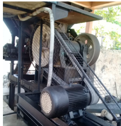
Figure 67: Construction waste crushing machine at COWAM Centre
